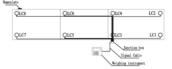
D、 Truck Scale with 4sets weighing platform(10 pcs load cell)
