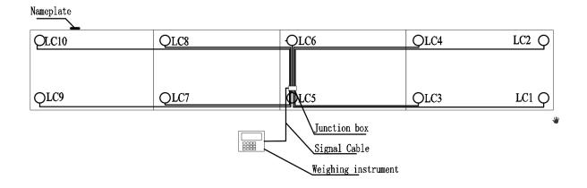
5.4.2 The connection between load cell and junction box
