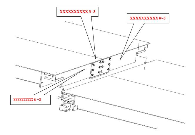
5.3.3.2 Installing weighing platform connecting plate
