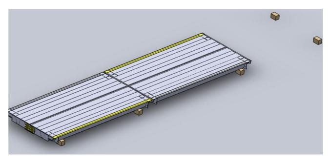
E. Lifting and placing third weighing platform, at the same time install the dowel pin to second weighing platform
