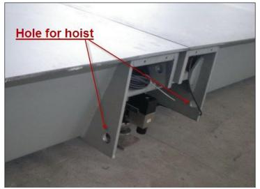
5.1.1 Using hole for hoist when truck scale hoisting
