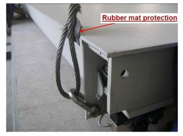
5.1.3 Scale body should be placed in a horizontal position
