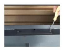
2. Lift one side of the Platform Scale (at least two people are required); then, insert the 4 glides provided in each threaded hold at the bottom of each comer.
