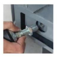
3.Place the platform scale at the desired location (room comers are recommended to prevent people form tripping). Adjust feet height with a flat screw driver to ensure the platform is leveled (see picture). Once the platform scale is leveled, tighten the nut on each foot glide.
