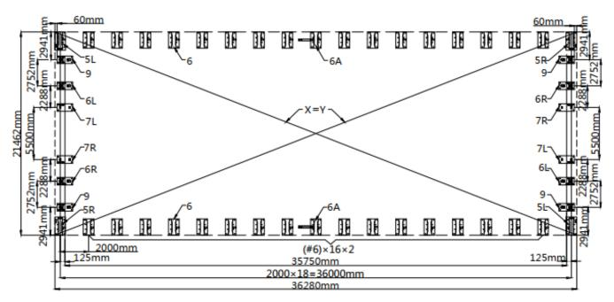
• Installation diagram of expansion bolt.
