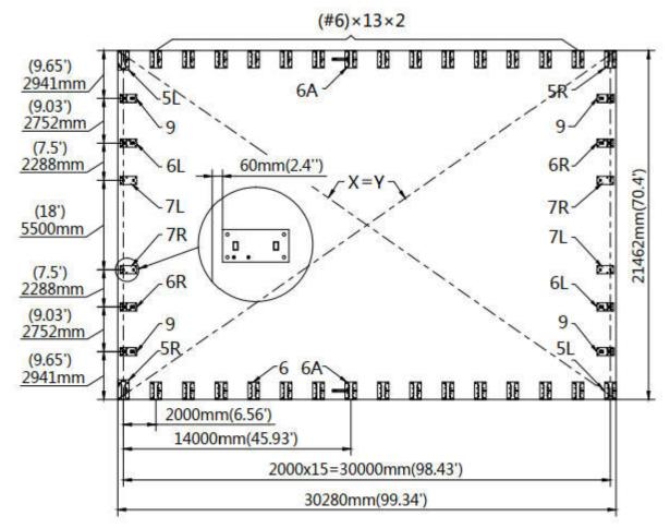
· Installation diagram of expansion bolt.
