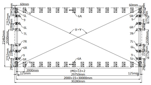
• Installation diagram of expansion bolt.
