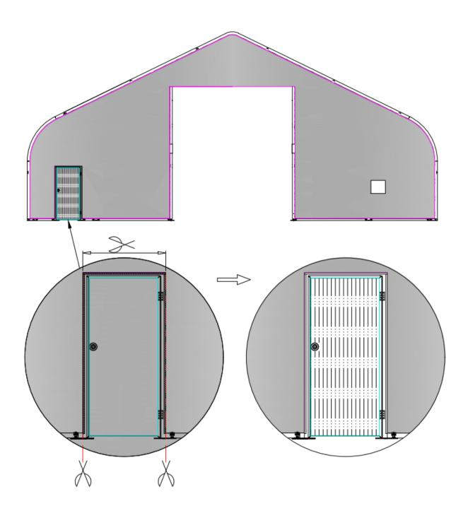
STEP 18: INSTALL THE FRONT DOOR METAL STRIP (THE FRONT AND REAR MOUNTING METHODS ARE THE SAME).
