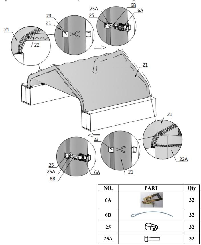
Step 21: Tension both sides of the top cloth with the tension device.
