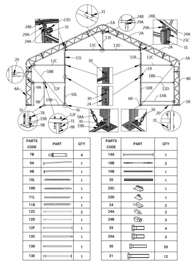
STEP 13 : FRONT AND REAR SMALL SIDE DOOR INSTALLATION.
