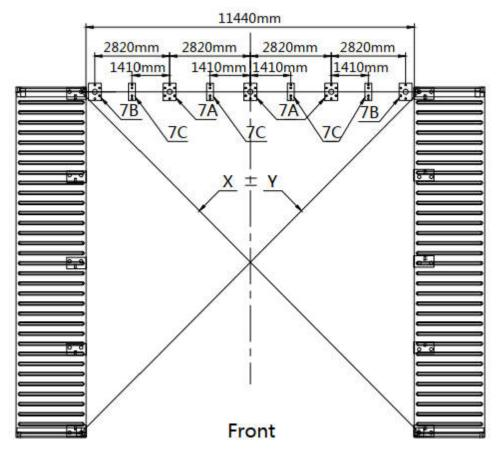
• Installation diagram of expansion bolt.
