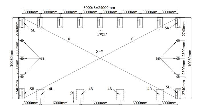
• Installation diagram of expansion bolt.
