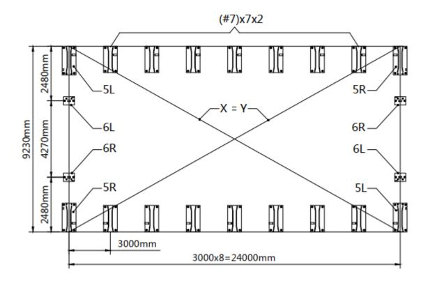
• Installation diagram of expansion bolt.
