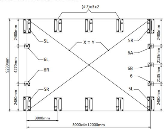
• Installation diagram of expansion bolt.
