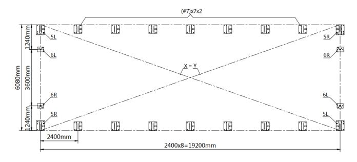
• Installation diagram of expansion bolt.
