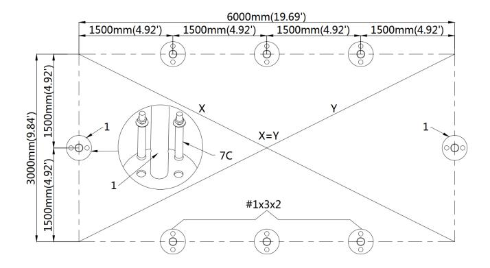
Installation diagram of expansion bolt.
