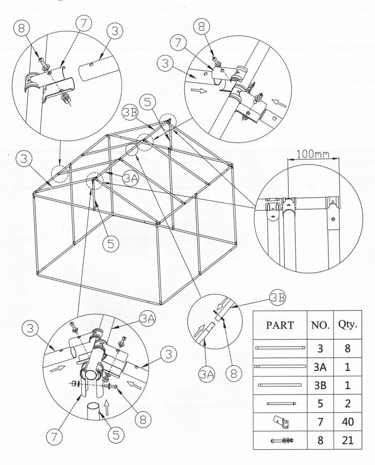
**Step 5 : The joints are fixed with self tapping screws**
