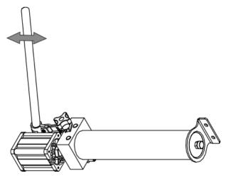
3. Continue pumping until the hydraulic fluid starts to come out from the end of the coupler tip and is free of air bubbles.
