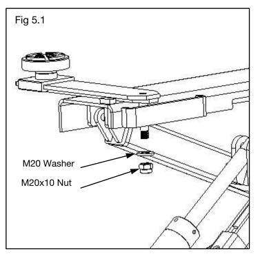
3. Tighten the M20-10 nut until the arm cannot pivot, then back the nut off until the arm is just loose enough to pivot freely. (See Fig.5.2)
