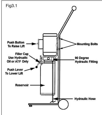
2. Remove plug from power unit and install the Straight Fitting into the power port on the Power Unit.
