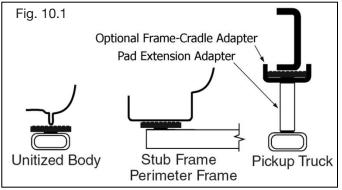
3. Some vehicles may have the manufacturer's Service Garage Lift Point locations identified by triangle shape marks on the undercarriage (reference ANSI/SAE J2184-1992). Also, there may be a label located on the right front door jamb area showing specific vehicle lift points.
