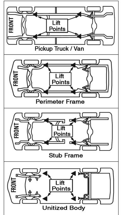
4. Position vehicle for proper weight distribution arms un- der vehicle to allow adapters /pads to contact at the manu- facturer's recommended pick up points. 5. If the specific vehicle lift points are not identified, or if the vehicle has additional or uniquely positioned payload, have a qualified person calculate the vehicle center of gravity or have the vehicle center of gravity determined at a vehicle scale. Load the vehicle with the enter of gravity midway between adapters.
