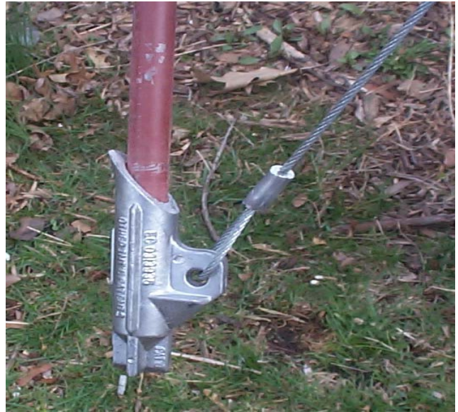
Drive Rod inserts into Anchor Head
