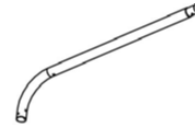
#4 / EUL-8002 (8) Lower Leg Pole w/foot swedged one end lower portion of leg poles #1, #4, #8, & #11
