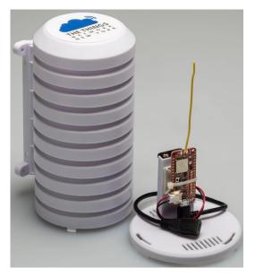
The long-range communication modules in the Model 4831-4832 are based on the MCCI Catena 4618 modules. MCCI provides a full Arduino board-support package and libraries allow rapid customization by system integrators, including an open-source LoRaWAN stack. ST Micro tools may also be used.
