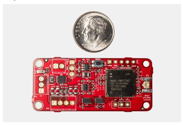
Based on the Murata CMWX1ZZABZ-078, the Catena 4801 is a great platform for RS485/Modbus based LoRaWAN investigation and deployment. It works well with The Things Network, myDevices, or any LoRaWAN 1.0 through 1.1 network in the 865 to 923 MHz range. It also works with Sigfox networks worldwide.
