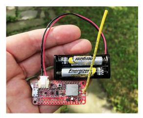
The MCCI Catena® 4618 is a complete single-board IoT device for LoRaWAN® technology projects.
