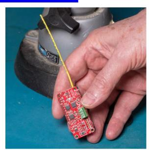
The MCCI Catena® 4470 Modbus Node for LoRaWAN® technology is a powerful open-source IoT device that integrates Modbus control with The Things Network. Based on the Adafruit Feather M0 system, the Catena 4470 is a ready-to-use platform for Modbus-oriented LoRaWAN 1.0 and 1.1 wireless IoT applications.
