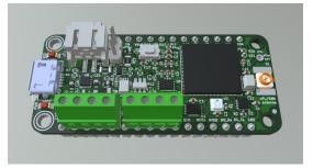
The Catena 4612 is pin-compatible with the Adafruit Feather M0 family of boards (with some limitations because the of functional differences between the STM32L082 CPU and the Atmel SAMD21 CPU used in the Feather M0).
