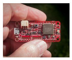
The MCCI Catena® 4612 is a complete single-board IoT device for LoRaWAN™ technology projects.
