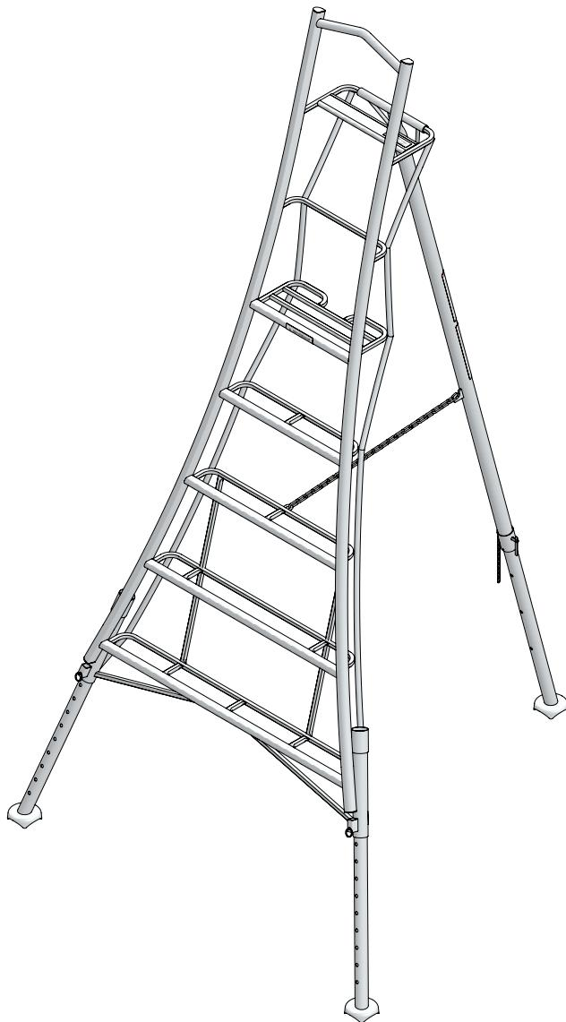
Check that the stiles and legs are not bent, bowed, twisted, dented, cracked, corroded.
