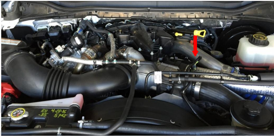
2017-2020 6.7L Powerstroke Charge Air Cooler Sensor Sensor is located on the top of the connector at the engine throttle body
