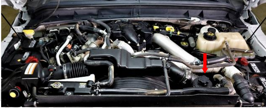
2011-2016 6.7L Powerstroke: Charge Air Cooler Sensor is located on the lower firewall side of the cold side intercooler tube.
