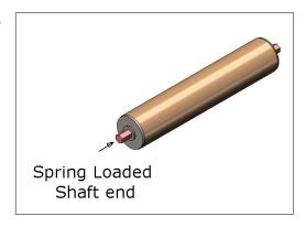
6. Compress the spring-loaded end of the shaft into the roller and release the shaft into the inboard slot.
