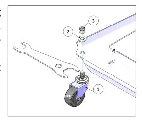
2. Install the **Flanged Swivel Casters (#4)** by inserting screws (#5) through the caster's flange and frame jaw, washer (#6) and by tightening the lock-nuts (#7) using a wrench, while holding the screws with an Allen key.
