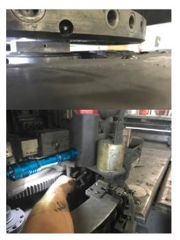
12). Jog station to punch. Remove sheetmetal and gently engage top and bottom alignment tool. I like to use a small pry bar to help this in. It should NOT take excessive force to engage. Rotating belt side to side while applying gentle pressure should allow the top to engage the bottom die.
