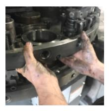
6). Reach under turret bushing and press the bushing up from station. If it needs some persuasion use a brass or aluminum punch to break it loose. Clean area thoroughly.
