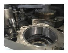
5). Remove 4 button head cap screws holding gear retainer plate, being careful to retain small shims under retainer. Remove and inspect retainer. Replace this if it appears damaged. Our part number CNC 3012.
