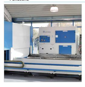
This is a highly effective unit, synchronized with the CNC machine, specially designed for extraction and filtration of dust and fumes generated during cutting operations. It starts and stops with the machine and shares fault signals.
