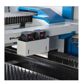
All guideways and racks are fully covered with high quality bellows, which protects against premature wear, while keeping away dust, slag and small cut parts.
