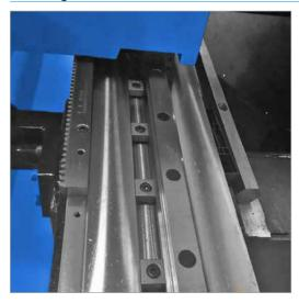
This laser cutting system features a gantry type construction with drives on both sides and a large working area that can accommodate most common plate sizes.
