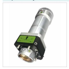
Cutting head features optimized design which includes closed loop water cooling for collimation and focusing lenses to prevent heating and increase stability when working with high power lasers.
