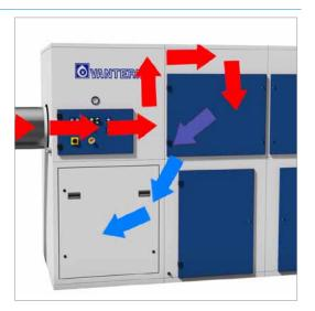
Standard features include a spark separator function. This has double functionality: to cool down the cutting residuum and to remove (by cyclonic separation) the bigger parts to prevent damage to the filters.
