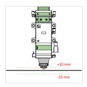
Focus lens can automatically change the position in the range of 25 mm (+10 ~ -10 mm) with adjustment accuracy of 0,05 mm. The user can set the focus continuously through the program to complete multiple paths of different thicknesses.
