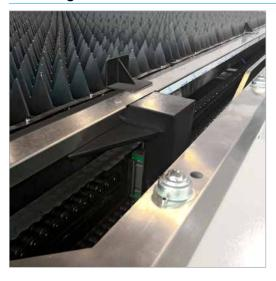
Workpiece weight is supported by brackets. After usage, they can be replaced via KNUTH, or can be machined by the customer. The DXF file for the brackets as well for the strips are already saved in the CNC control.
