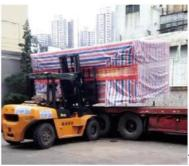
The forklift truck should unload the machine like the image (left).
