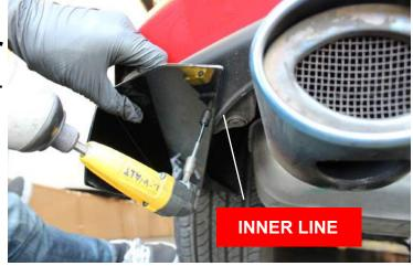
\*NOTE\* - INNER LINE is a guide for the diffuser to be side by side with it, will not past it, nor be on top.
