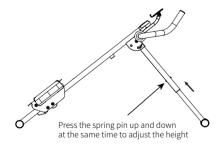
STEP 5: Movement mode: A slide up B slide down
