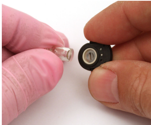
Figure 27: Reinstalling the Electrode Lamp
