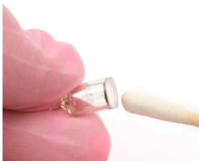
Figure 26: Polishing the Electrode Lamp Window
