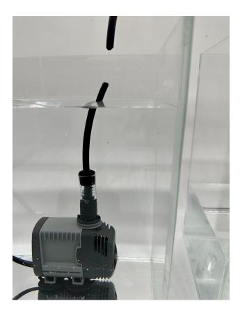
We are going to install the anti siphon bulkhead here and care must be taken to make sure the hole in this fitting is never submerged. During operation water will be coming out of this hole, adjust the nut so it covers the hole to prevent spray if you are not installing through a lidded container. When the pump shuts off, air will enter in this small hole and prevent a siphon from forming.
