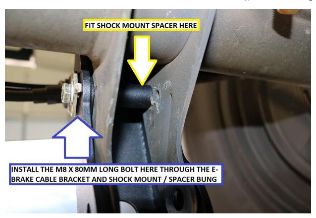
12) Next, install the new lower shock bolt included with the kit. This is simply used to hole alignment of the bracket while we snug the other mounting bolts.
