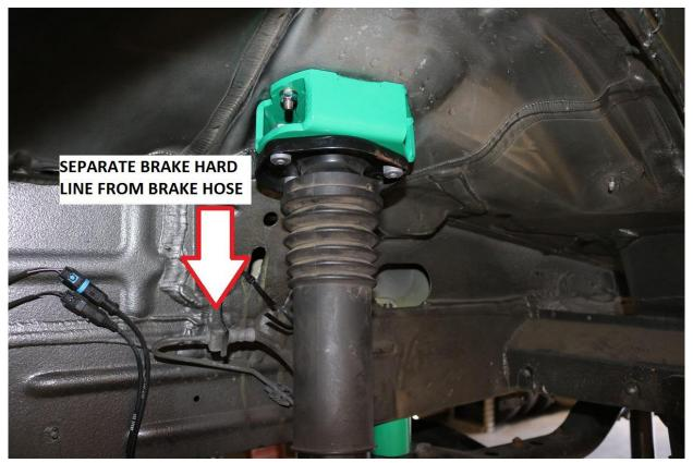
79) Install the front brake line drop bracket as shown below. Use the M12-1.50 x 25mm long bolts provided in the kit. Use a washer under both the nut and the head of the bolt.
