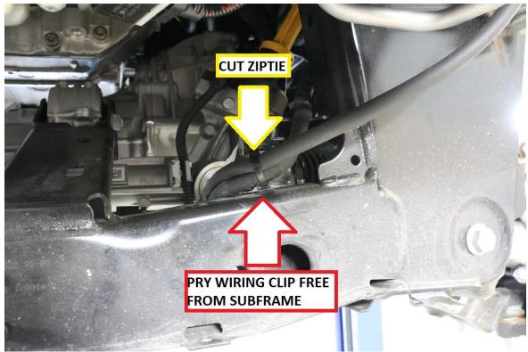
27) Locate the wiring retention clip on the inside of the suspension subframe near the inner tie rod joint on the driver side. Again, use an automotive trim removal tool to separate the retention clip from the subframe. See image below for reference.
