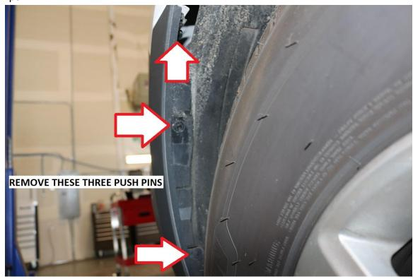
13) Locate and remove the three plastic nuts securing the front half of the inner fender well liner to the chassis. Use a 10mm socket for removal.
