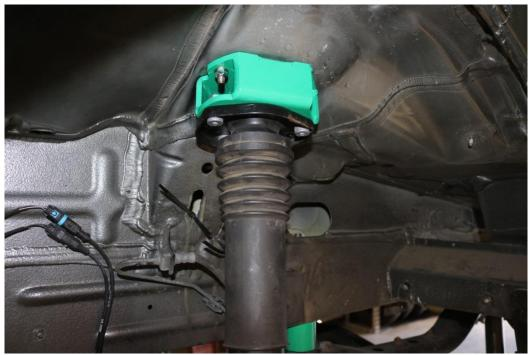
58) With all bolts installed and snug, torque to 21 ft-lbs (28 N.m)
