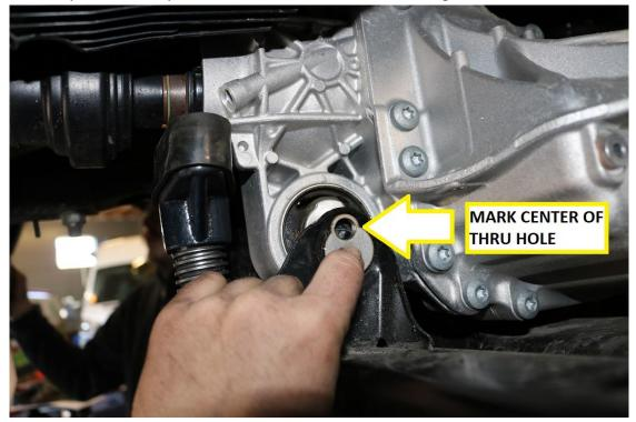
70) Center punch the marked hole and drill with a ¼" pilot hole to start. Just drill thru the one side of the bracket with the pilot drill.
