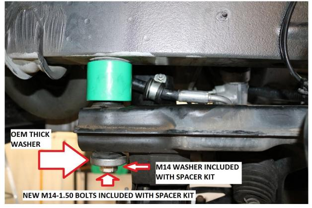
42) Snug all 6 bolts but do not torque at this time. Final torque will occur once the motor mount spacers are installed and the engine / transmission support jacks & jack stands can be removed.
