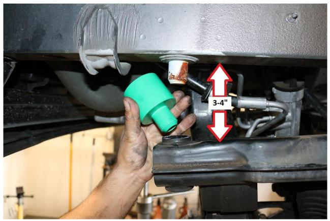
41) Install all 6 spacers in their corresponding locations and raise the sub frame into place.
