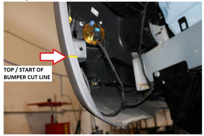
100) From the line marked in the previous step, continue cut line down so it is tangent with the bottom outer push pin hole in the front bumper cover. See image below for reference.
