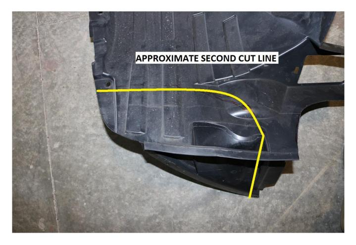
103) Example of a finished cut front inner fender liner is shown below.
