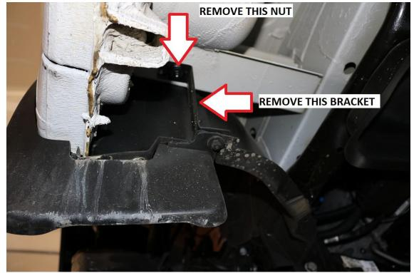
93) Remove and retain the clip-on nuts which secured the mudflap to the rear of the front fender.
