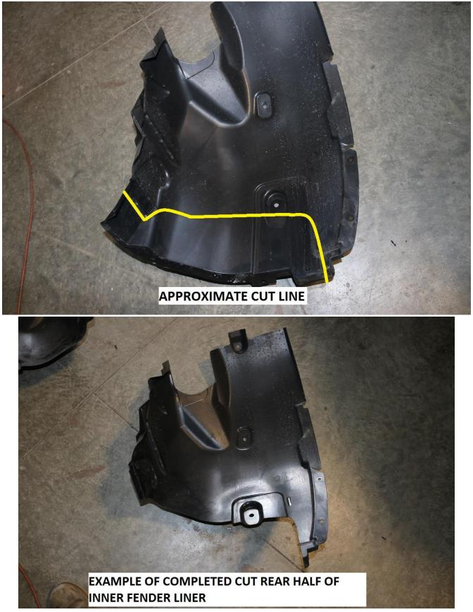
Install trimmed fender liners and mudflap as shown below.
