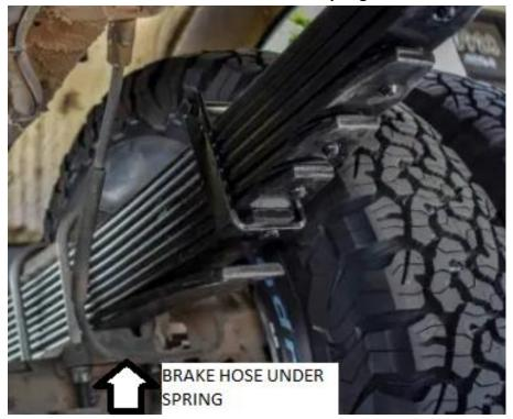
14) Once the springs are rotated into position. Install the forward spring bolt in the spring hanger slightly, install one of the provided washers between the spring and spring hanger. Push the bolt though the washer and into the spring. Install the second washer between the spring and hanger and push the bolt all the way through. Install the nut but do not tighten at this time.
