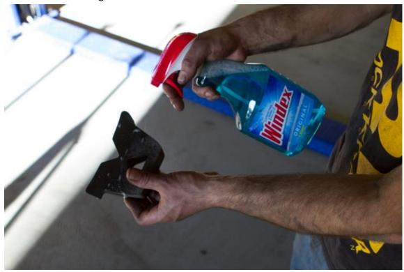
26) Install bump stop into the drop bracket. Install one edge at a time. Bend the bump stop in the middle to get the second side started. Installation can be tricky as the bump stops fit very tightly both in the factory location and in the drop brackets.
