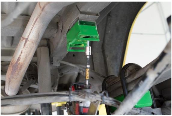
24) Use drill / driver to snug bolts into place. Do not fully tighten using drill / driver. Torque bolts to 13 ft-lbs (17 N.m).
