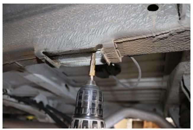
23) With both holes drilled, positions the bump stop drop bracket in place and secure it to the chassis using the  $5/16-18 \times 1''$  long thread cutting screws included with the kit. Use a nut driver or drill with a 1/4'' bit adapter and a 1/4'' socket to install the screw. Try to keep the drill / driver as straight as possible when cutting the threads.
