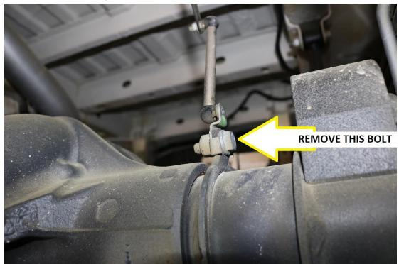
5) Support the axle and disconnect the lower shock bolt. Use a 21mm socket and wrench for removal. Once the shock is removed, allow the axle to hang freely again. Note that the springs will limit the downward travel with the shocks removed.
