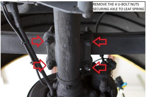
8) Lower the rear axle on the driver's side until there is approximately 3" (75mm) between the axle spring perch and the bottom of the leaf spring. Remove the factory lift block for the time being. The factory lift block will be re-installed with the new leaf springs.
