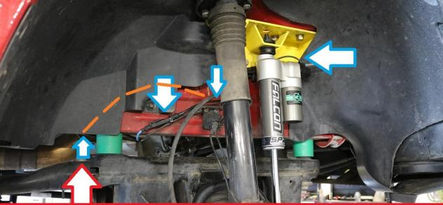
NOTE THIS VAN IS EQUIPPED WITH A VC 2" STRIKER LIFT KIT. VANS WITHOUT A LIFT KIT INSTALLED WILL HAVE THE WIRING EXIT TO THE WHEEL WELL IN THIS LOCATION. FOLLOW THE DASHED ORANGE LINE FOR ROUTING BEHIND THE FENDER LINER
