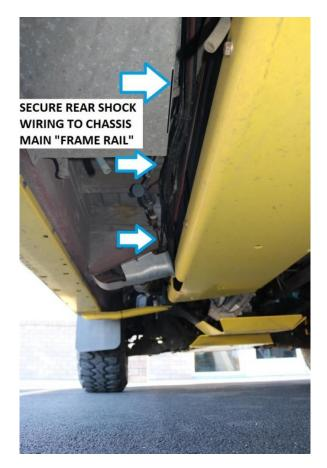
20) Split the driver / passenger side rear shock wiring at the crossmember where the rear brake lines are run. Plug the shocks in and loop up any excess wiring at the chassis.
