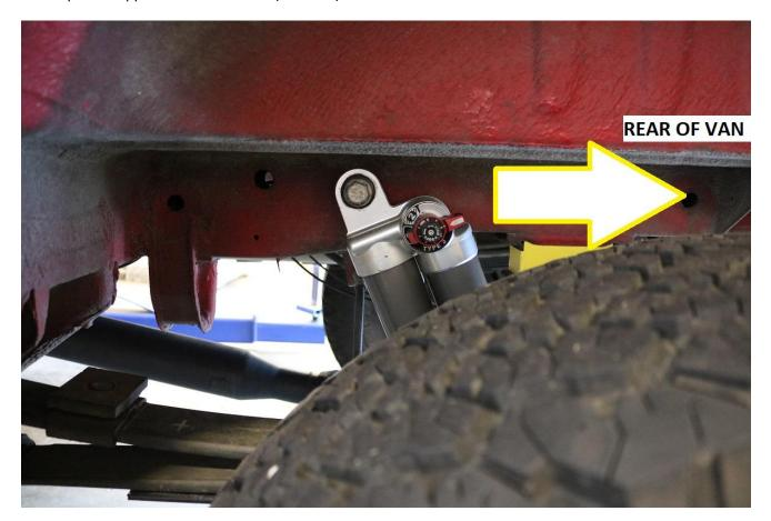
6) With the top of the shock bolted into the upper mount, ensure the shock shaft is extended out all the way. Adjust the SP2 mode adjust by rotating the shaft 360 degrees in the direction as specified below for the corresponding van weights:
