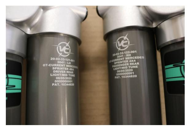
4) Install the shock into the upper mount using the factory bolt and included spacer washer as shown. Use a dab of red Loctite on the threads of the upper bolt.
