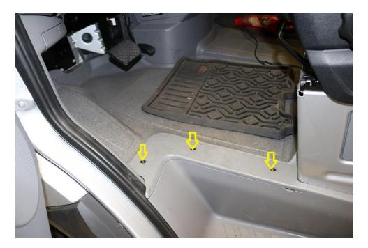
b. For 2019+ VS30 models, locate the two T25 Torx screws securing the floor mat cover to the door sill. Remove these screws and remove the driver side floor mat.
