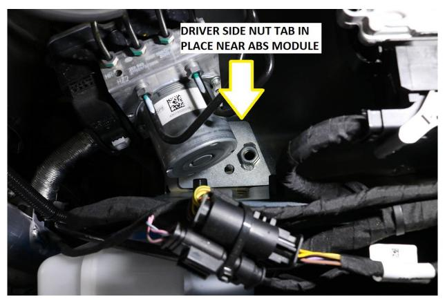
18) Install the upper shock bracket on the driver side (left hand). The mounts are left and right specific and can only be installed one way. For the nut tab locations, use a lock washer under the bolt head, followed by a flat washer as shown below.
