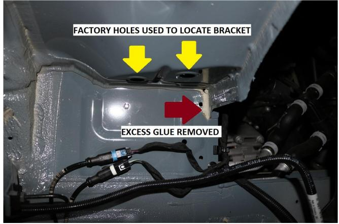
30) Touch up any bare areas of metal with paint to prevent corrosion.
