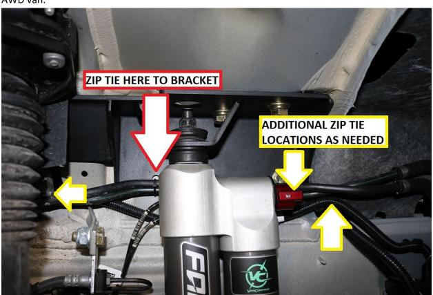
36) Vehicles equipped with the HD rear A/C option will require the routing of A/C lines & fitment of shock absorber to appear as shown in the image below.
