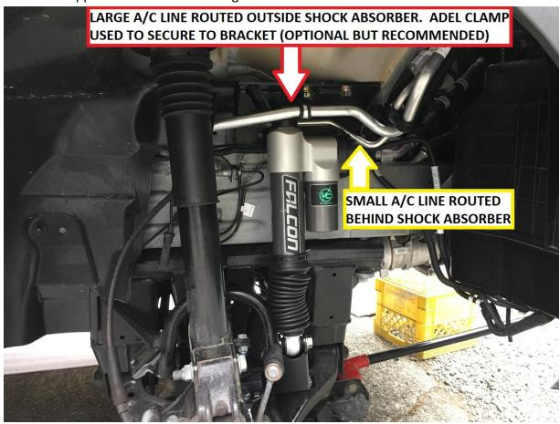
37) With brackets installed, install the shocks into the lower mounting bracket first. Use the  $9/16-12 \times 3.0$ " long bolt provided in the kit and install as shown below. Use a washer under the bolt head and stover nut.
