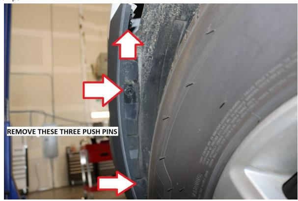
7) Locate and remove the three plastic nuts securing the front half of the inner fender well liner to the chassis. Use a 10mm socket for removal.
