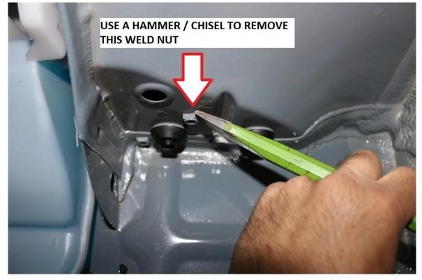
17) Once the weld nut is removed, drill out the hole using a 3/8" or 10mm drill bit.
