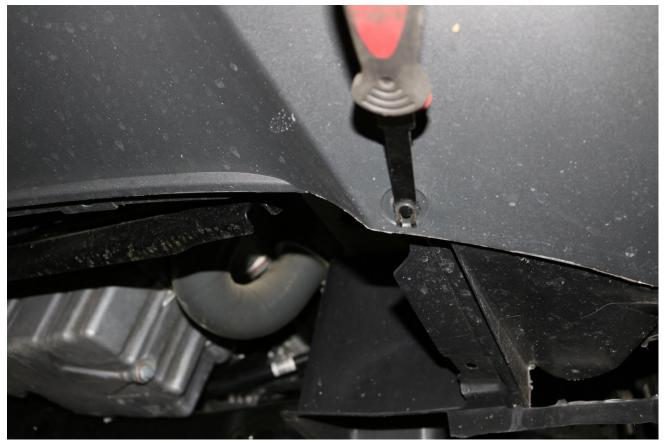
6) Next, on the inside of the fender well, remove the three push pin fasteners near the outer lip of the bumper.
