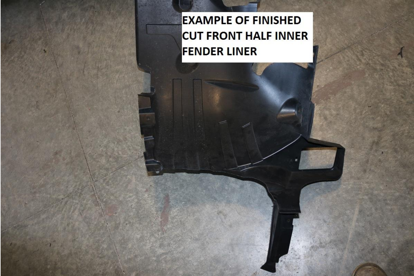
89) Example of a finished cut front inner fender liner is shown below.
