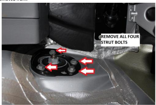
24) The passenger side upper strut bolts can be accessed by pulling up the floor jack / tool kit cover panel in the passenger footwell. Refer to your owners manual for access if not already familiar with this procedure.
