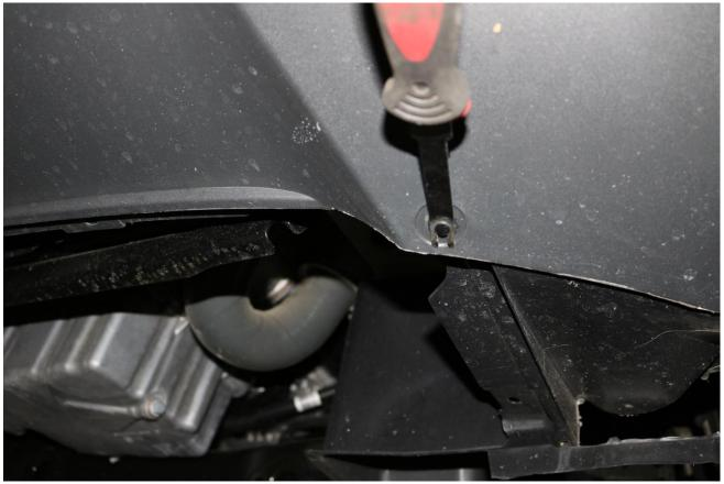
12) Next, on the inside of the fender well, remove the three push pin fasteners near the outer lip of the bumper.
