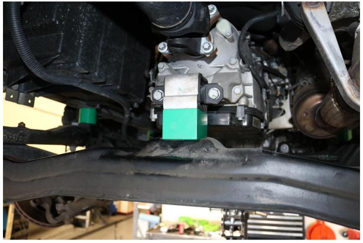
41) Install the M8-1.25 x 70mm long bolts provided in the kit and snug all hardware finger tight. Final tightening will occur once the motor mount lift spacers are installed.
