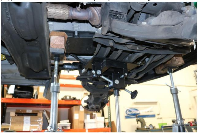
33) The ABS / ESP wiring barb retention clip may need to be pried out of the sub frame for installation of the spacers. Use an automotive trim removal tool to separate the clip from the sub frame.
