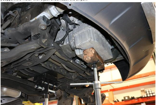
26) Remove the motor mount bolt on both the driver and passenger side with a 16mm socket / wrench.
