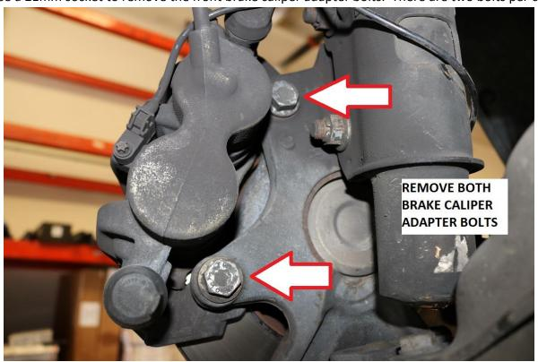
20) Remove the brake caliper from the rotor and secure up out of the way. Do not allow the caliper to hang by the brake hose.
