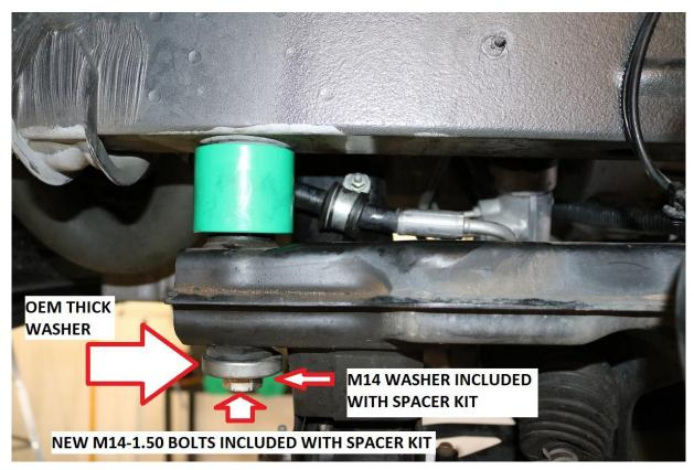
39) Snug all 6 bolts but do not torque at this time. Final torqueing will occur once the motor mount spacers are installed and the engine / transmission support jacks & jack stands can be removed.
