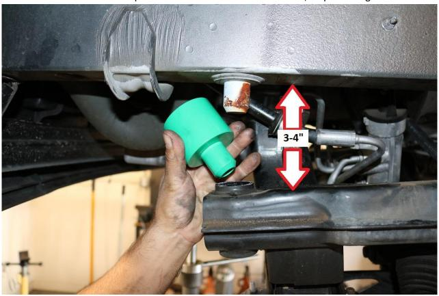
38) Install all 6 spacers in their corresponding locations and raise the sub frame into place.
