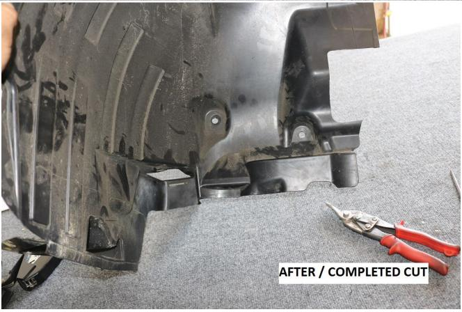
60) If larger tires are being installed, specifically 265/70 or larger, trim the rear half of the fender liners as shown in the images below.
