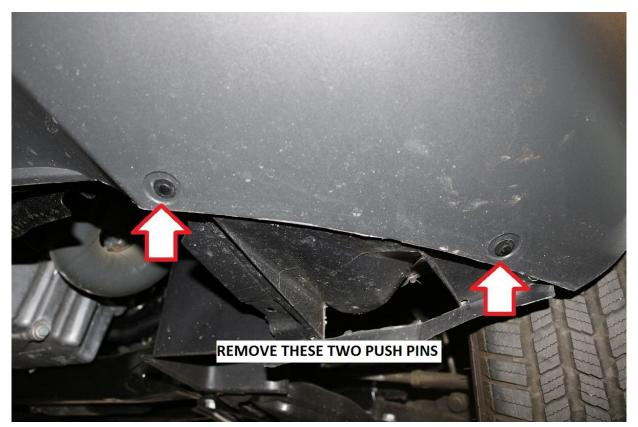
11) Use an automotive trim removal tool to pry up under the head of the push pin prior to prying under the body of the fastener to fully remove it.
