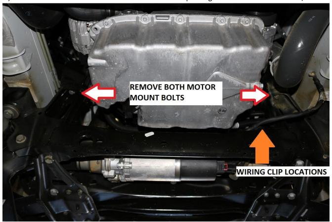
27) Locate the wiring for the electric power steering rack on the driver side (left side) of the suspension sub frame. The orange arrow in the previous photo shows the approximate location of this wiring. Once located, pry the two barbed wiring clips out of their mounting holes so the wiring does not become strained when the lift is installed. See image below for reference.
