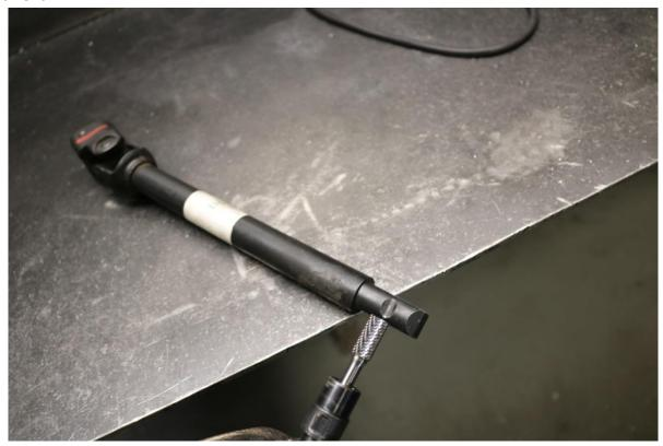
90) Once the pinch bolt can easily be installed, paint any newly exposed areas of metal to prevent corrosion. Assemble the steering shaft extension onto the steering shaft as shown below. Use a small dab of blue Loctite on the threads of the socket cap screw and torque to 18 ft-lbs (24N.m) using a 6mm Allen wrench.
