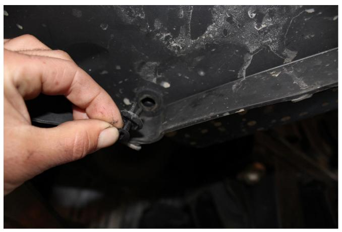
21) Next, on the inside of the fender well, remove the three push pin fasteners near the outer lip of the bumper.
