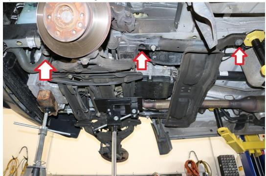
45) Prepare the spacers and new sub frame attachment bolts. The image below shows where each bolt / spacer is designed to be installed. It is critical to use the correct bolts / spacers in their corresponding locations.
