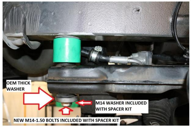
49) Snug all 6 bolts but do not torque at this time. Final torqueing will occur once the motor mount spacers are installed and the engine / transmission support jacks & jack stands can be removed.
