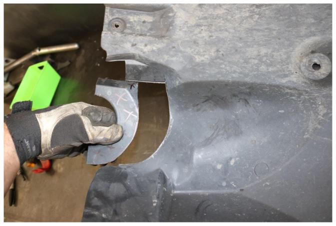
77) Again, if fitting 315/75/16 (35") tires, trim the rear half of the inner fender well liner as shown below.78) Measure 1.50" down from the rear center mounting stud location and mark a line. See image below for reference.
