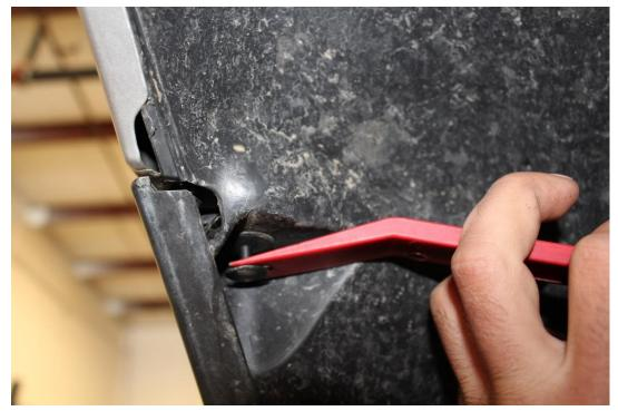
23) Locate and remove the two plastic nuts securing the front half of the inner fender well liner to the chassis. Use a 10mm socket for removal.
