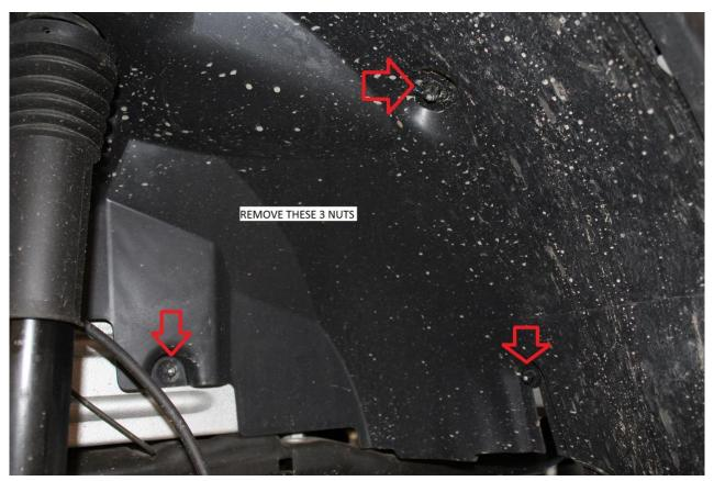
25) Lastly, remove the upper nut which secures both the front and rear half of the inner fender well liner to the chassis. Again, use a 10mm socket for removal.
