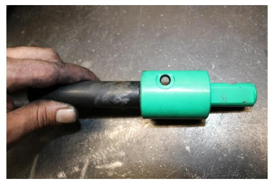
89) If the notch needs to be modified to allow for the bolt to be installed, use a small die grinder with burr bit or a 4-1/2" angle grinder with metal grinding wheel. Remove as little material as possible to allow fitment.
