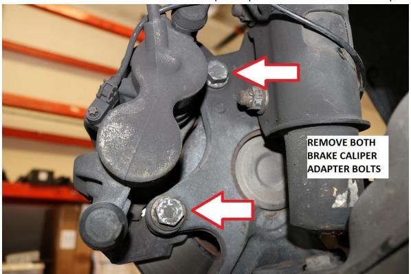
14) Remove the brake caliper from the rotor and secure up out of the way. Do not allow the caliper to hang by the brake hose.
