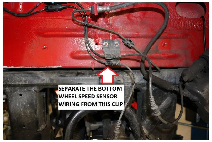
42) Separate the barbed wiring clips from the chassis in the locations denoted in the image below. Make sure this wire is free from the suspension sub frame prior to performing sub frame drop.
