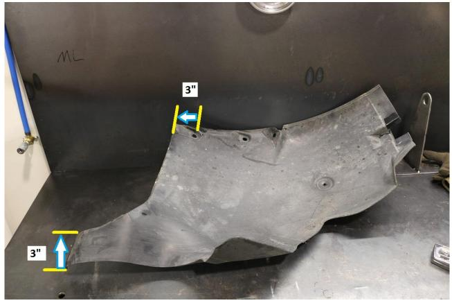
76) The rear half of the fender well liner trimming is very similar. Again, see the images below for reference.
