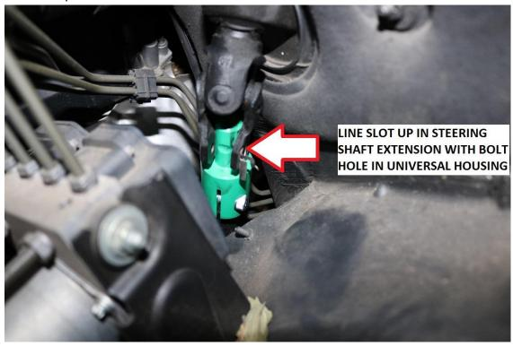
93) Install the bolt, retaining clip and nut removed in step 6 back onto the steering shaft. Use a 13mm socket / wrench and torque to 18 ft-lbs. (24 N.m)
