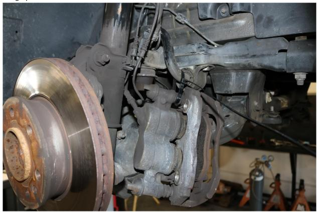
15) Raise the lower control arm about 3/8" (10mm) to remove tension from the strut. Use a 21mm socket to remove the 2 bolts securing the strut to the steering knuckle.
