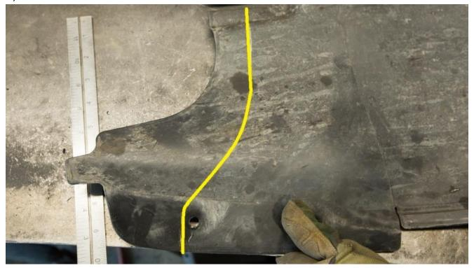
81) Re-install the fender well liners in the reverse order of removal. The trimmed liners should appear as shown below.
