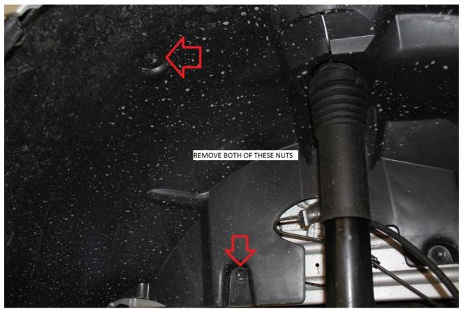
24) Locate and remove the 3 plastic 10mm nuts securing the rear half of the inner fender well liner to the chassis.
