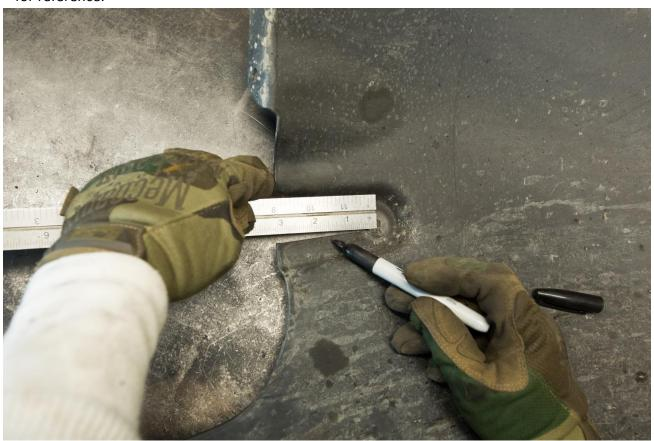
79) Mark a line just below the lower mudflap mounting hole on the outer edge of the fender liner.
