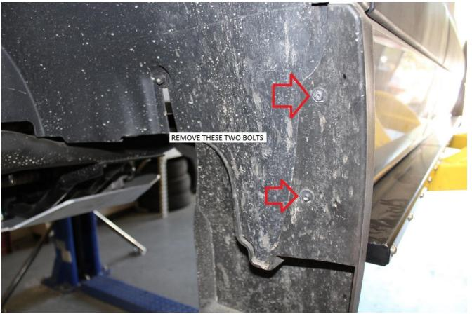
30) Pull the mudflap out away from the body so the inner fender well liner can be pulled free from behind it. Again, pull the inner fender well liner out from underneath the lip of the fender. And pull the liner away from the bottom stud.
