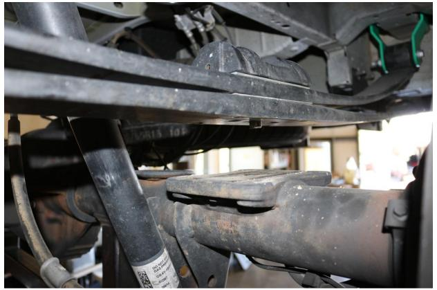
10) Install the lift block and new U-bolts included with the kit. Use a new M14-1.50 nylock nut and washer. Snug all bolts and repeat steps 4-8 on the passenger side.
