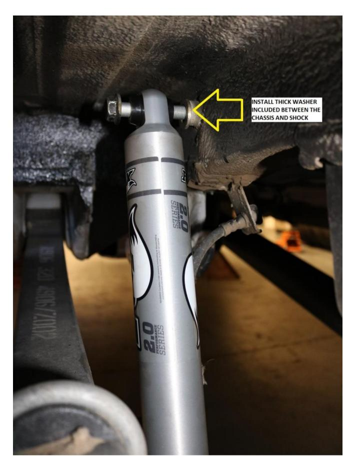
4) Snug upper shock bolt using a 21mm socket / wrench. Do not fully tighten at this time though.
