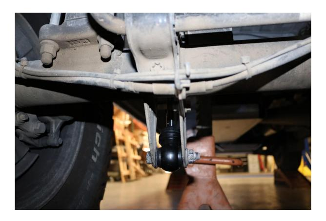
6) Attach the reservoirs with the provided clamps. Position them as shown below. Be sure the reservoir will not come into contact with the axle as the suspension compresses and is not rubbing the brake hose. Use a ¼" allen wrench to tighten.
