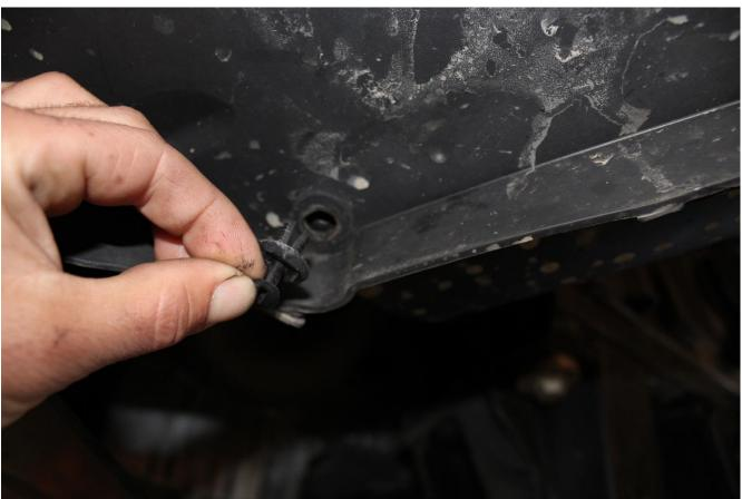
7) Next, on the inside of the fender well, remove the three push pin fasteners near the outer lip of the bumper.
