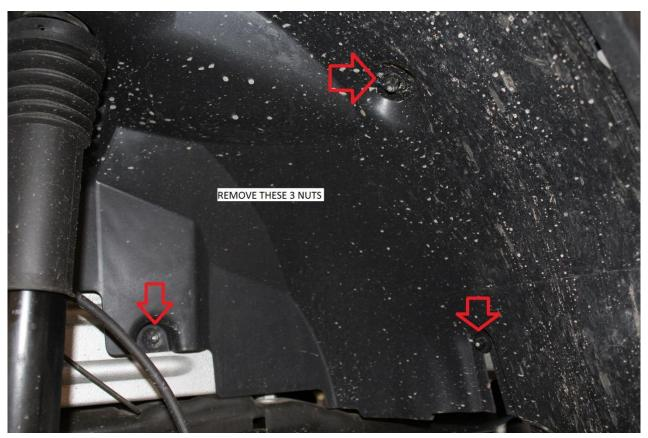
11) Lastly, remove the upper nut which secures both the front and rear half of the inner fender well liner to the chassis. Again, use a 10mm socket for removal.
