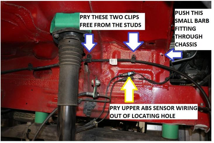
36) Cut / grind smooth the threaded studs where the upper wiring was attached to. See the following two images for before / after reference images.
