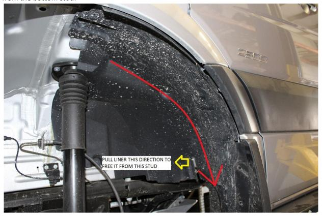
14) The liner should now be able to rotate down and out the direction denoted above with the large red arrow.
