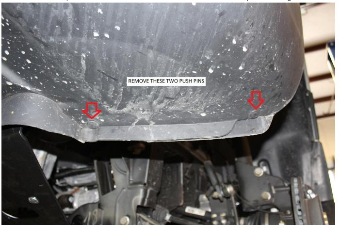
5) Using an automotive trim removal tool, pull up the head of the push pin. In most instances, the entire push pin assembly will come out.
