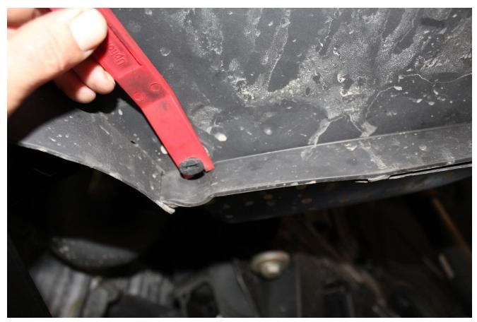
6) Using the same automotive trim removal tool, pry up under the head of the push pin body to fully removal the fastener.
