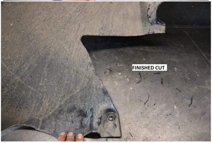
46) Trim the rear half of the factory inner fender well liner as shown in the images below.
