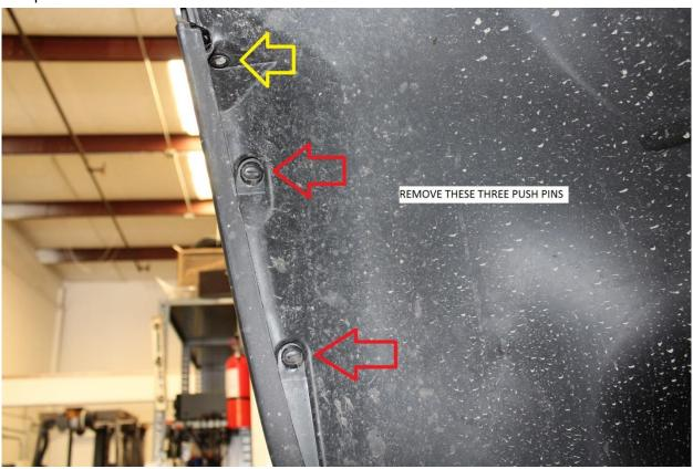
8) Note, the bottom two fasteners (denoted with the red arrows). The upper fastener (denoted with the yellow arrow) is a slightly larger push pin, take note of the different head style and be sure to reinstall in the same location during reassembly.
