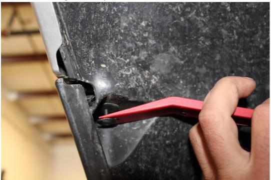
9) Locate and remove the two plastic nuts securing the front half of the inner fender well liner to the chassis. Use a 10mm socket for removal.
