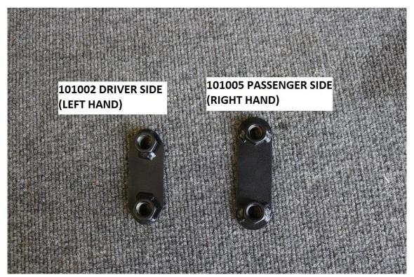
23) Install the nut tab from the engine bay so the threads are centered over the holes shown in the image below. Install so the plate is flat against the body, the welds on the nuts should be on the top side.
