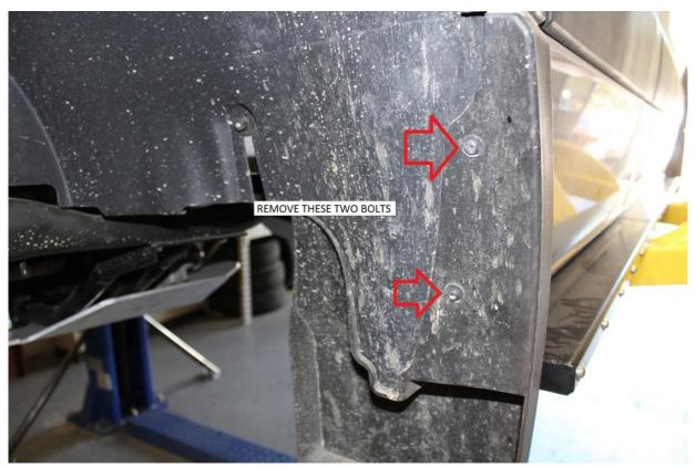
13) Pull the mudflap out away from the body so the inner fender well liner can be pulled free from behind it. Pull the inner fender well liner out from underneath the lip of the fender and pull the liner away from the bottom stud.
