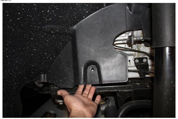
16) Next pull the inner fender well liner away from the bumper and out from under the fender lip until it appears as shown.
