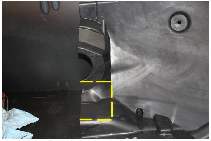
47) Re-install fender well liners and zip tie upper ABS / wheel speed sensor wiring in place as shown below.
