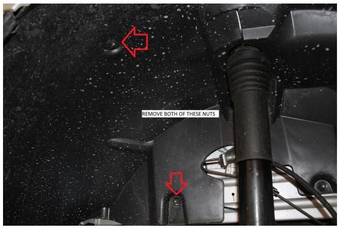
10) Locate and remove the 3 plastic 10mm nuts securing the rear half of the inner fender well liner to the chassis.
