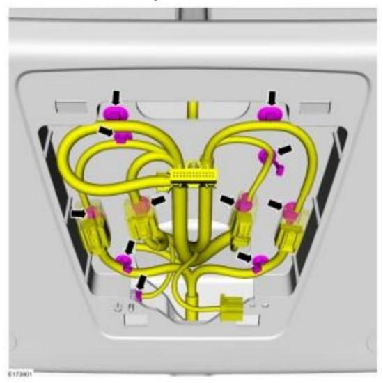
7) With the center wiring un-plugged and free from the overhead console, peer through the center opening and locate the 7mm bolt head which secures the center of the overhead console to the roof. Remove this bolt with a 7mm socket.
