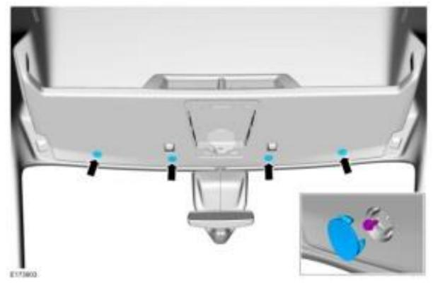
11) At this point, have a helper come support the overhead console and remove the 4 outer bolts near the upper grab handle at the outer edge of the overhead console. See image below for reference location of the bolts. Use a 7mm socket for bolt removal.
