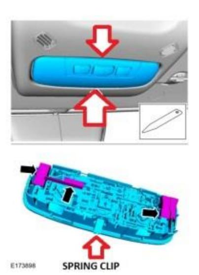
4) Look through the holes of the overhead console storage bins and locate the two tabs / plastic fingers which secure the overhead console center assembly. Release these two tabs by pushing forward and down so the overhead console center assembly can rotate downwards. These two tabs are stiff and require a good amount of pressure to release them. Use a large flat blade screwdriver to aide in depressing the tabs.
