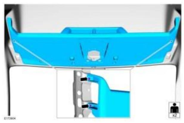
12) At this point, two helpers or a vertical support tool will be needed to fit the overhead main shelf to the vehicle.
