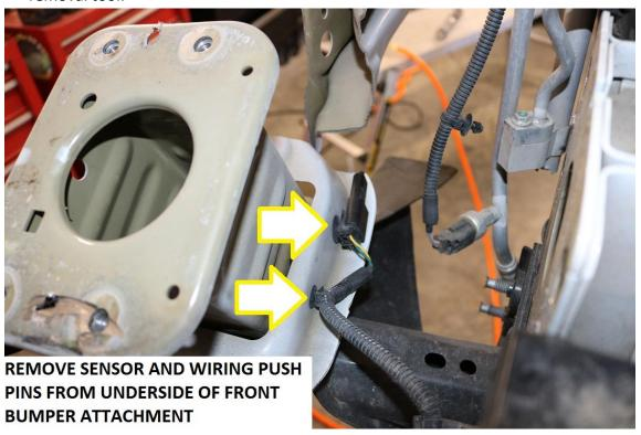
18) On newer vans equipped with active braking or adaptive cruise control, there is a radar sensor located behind the factory bumper.
