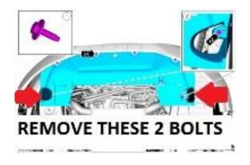
7) Next, remove the front license plate mount if equipped. On this vehicle, the license plate mount was secured with two 5/16" bolts.
