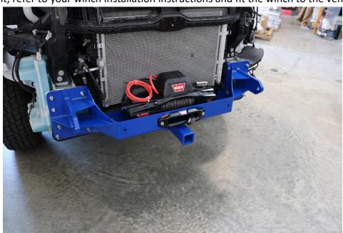
34) Reconnect / secure all wiring. Connect the wiring back to the A/C sensor unplugged in step 31. Connect wiring through the access hole in the winch mount as shown below.
