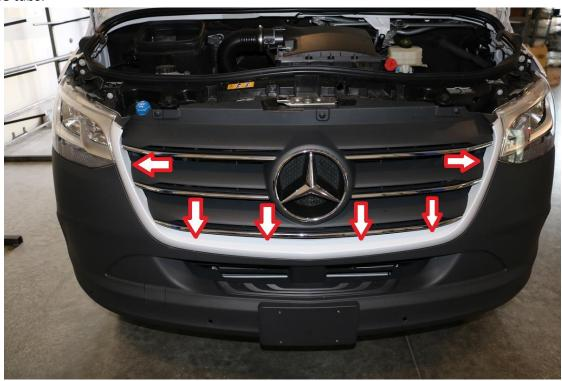
3) Once these tabs are located, push down on them and gently pull the bottom of the grille away from the van and it should come free from the vehicle. We have found a long flat nose screwdriver to work well as a tool to push down on the tabs.
