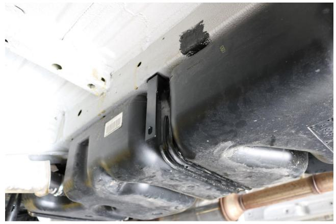
6) For the front angled brackets, line the inside edge up with the corner of the factory fuel tank straps.
