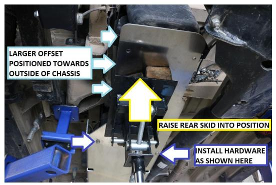
15) With the front bolts of the rear skid in position, install the rear bolts which attach to the skid to the rear hangers. Again, use a washer under the bolt head and start a flange nut on the top side.
