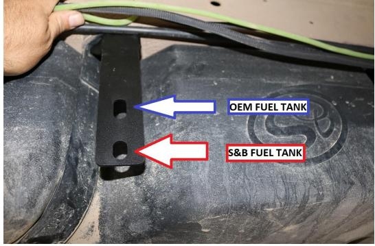
10) Install the 7/16-14 x 1.0" long hex head bolts included with the kit to attach the skid plate to the brackets. Use a washer under the bolt head and secure the brackets to the skid plate with the flange nuts provided. Skid plate should be installed as shown below.
