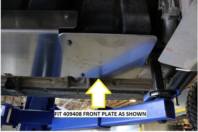
13) Installation for an OEM fuel tank or the S&B 40 gallon (part number: 10-1026) is now complete.
